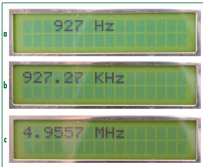
Figure 4. The units used for displayed switch automatically between (a) Hz, (b) kHz, and (c) MHz, according to the input frequency.
